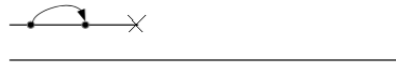
Figure 3: An execution that satisfies Total Order Broadcast but does not satisfy Uniform Reliable Broadcast .
